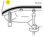
3. Gently insert and tighten bolts to keep oil pan gasket and oil pan in place
